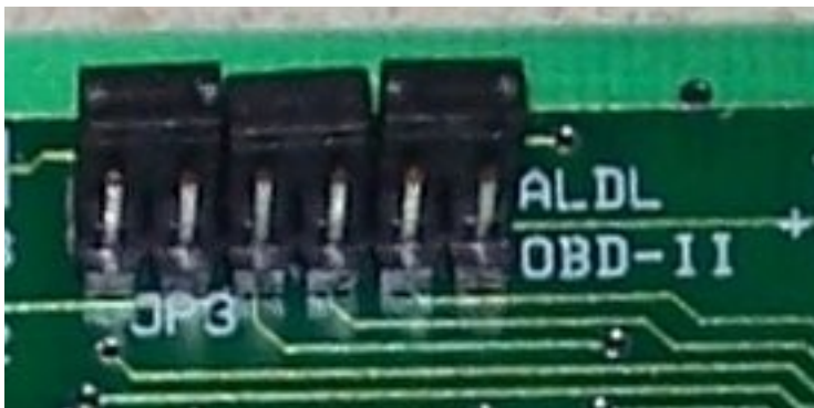
Illustration 3 - JP3 jumpers in ALDL mode (1G DSMs)
