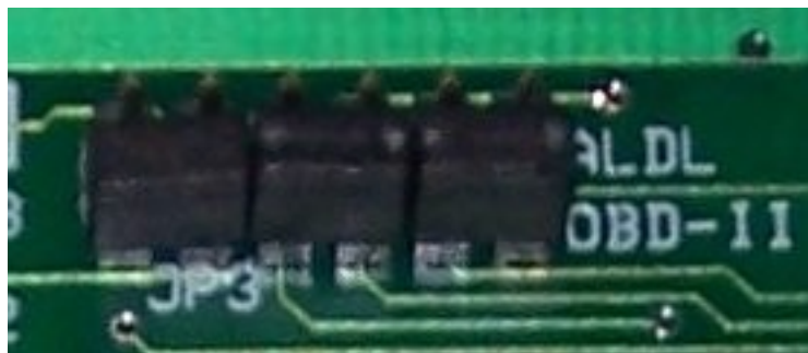
Illustration 4 - JP3 jumpers in OBD-II mode (2G DSMs and the EVOs)
